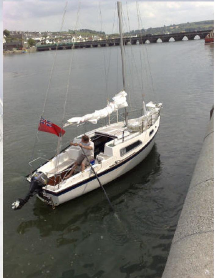
rope to the stern rail and the other with a tail wrapped on the winch. The knot is just a round turn and bowline so it can easily be undone and slid up and down the shaft to get the oar length correct. The tail on the winch ensures the lines stay tight. To protect the gunwale is yet another piece of UPVC held with tape. This is all easily removed when not needed
